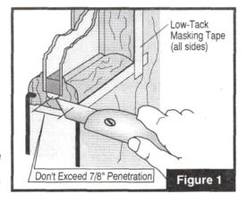
5. Remove any remaining glass or sealant material from the exterior surround and thoroughly clean glazing seat.
